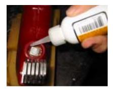
Applying glue carefully on switch cover Seat
